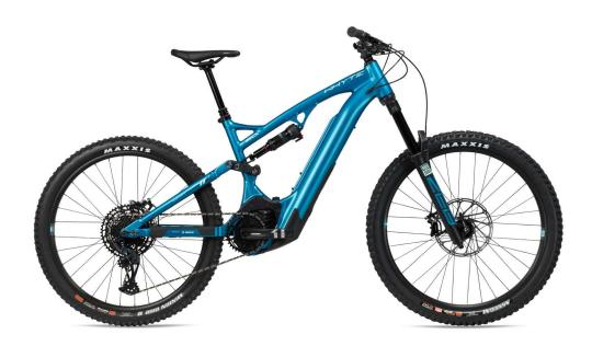
The E-160 S is available in 5 sizes from XS to XL. The RockShox ZEB 38mm stanchioned forks perfectly complement our proprietary OTO geometry for maximum steering control, and powerful Guide RE brakes keep the easy speed under control.
